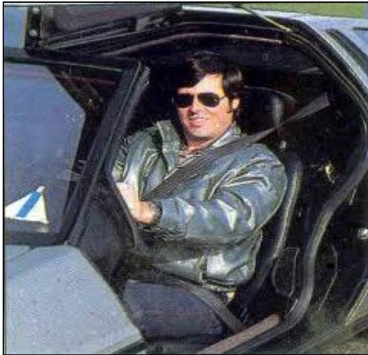
DeLorean's gull-wing doors (above and right) lift easily on gas struts, allow good entry into the spacious cabin
